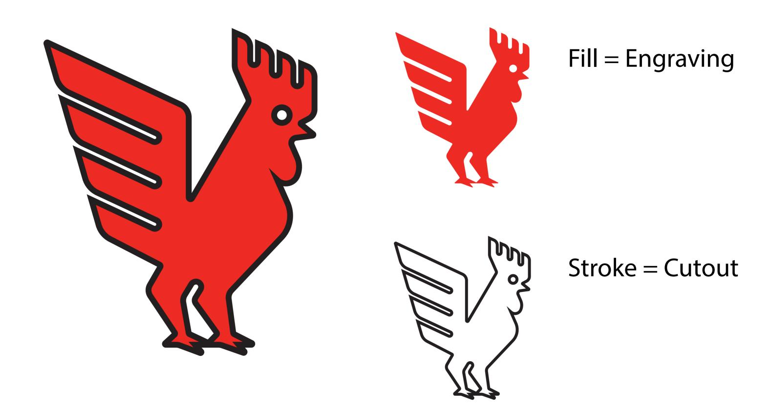
When using basic SVG support, the strokes in this rooster design should be exported in three files if you want the cutout between the legs and around the eye to work.
